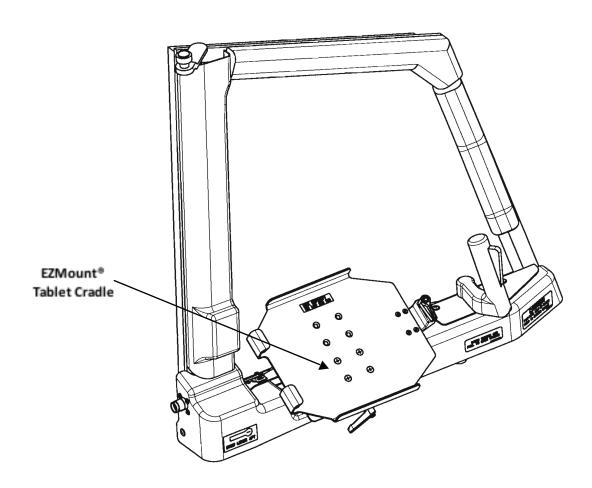
FIGURE 1 - CAPTAIN SIDE WINDOW MODIFIED WITH EZMOUNT™ TABLET CRADLE (8.0" X 10.7")
